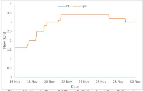
Figure 38. Hourly Flows PWR vs. Spill (Lookout Dam Tailrace).
