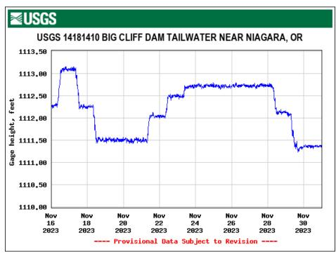
Figure 11. Gauge height (ft); below Big Cliff Dam.
