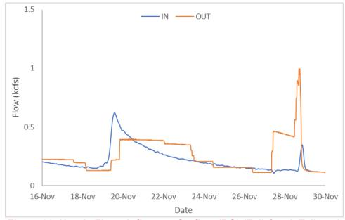
Figure 32. Hourly Flows Inflow vs. Outflow (RO) (Fall Creek Tailrace)
